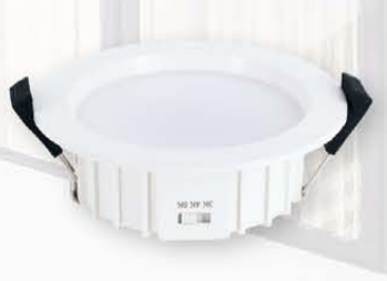
8W Downlight 110mm 3CCT 90mm Cut Out 3000K/4000K/5000K, 800-900 lumens. ADLED110R-3T - Q5071020
